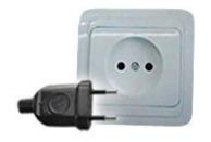
The "Europlug" is used in Southeast Asia as well. It is a two-wire plug, ungrounded, with two round, 4 mm pins. It will work with any socket that accepts 4 mm or 4.8 mm round contacts spaced 19 mm apart.
